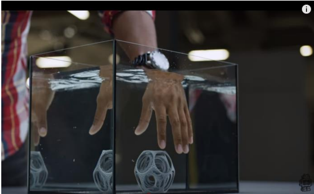
Figure 3: YOUTUBE video showing pre – and post processing of FDM parts on the Ultimaker 3D printer (Source: https://www.youtube.com/watch?v=0ENgGkPP94w )
