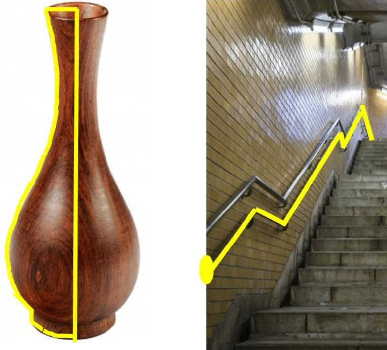
Figure 4: Example of everyday products which can modelled with revolve and sweep in CAD
