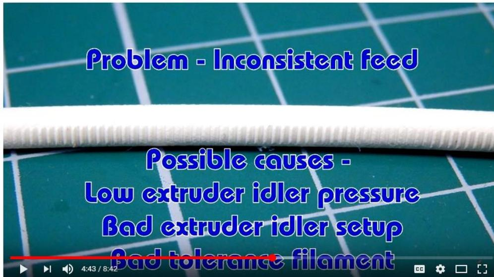
**Figure 2** – YOUTUBE video showing 3DPrinting Tips & Tricks Delamination of layers due to poor extrusion
