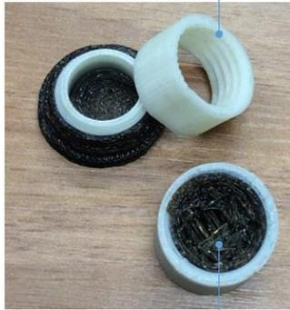
Support material required for the internal thread
